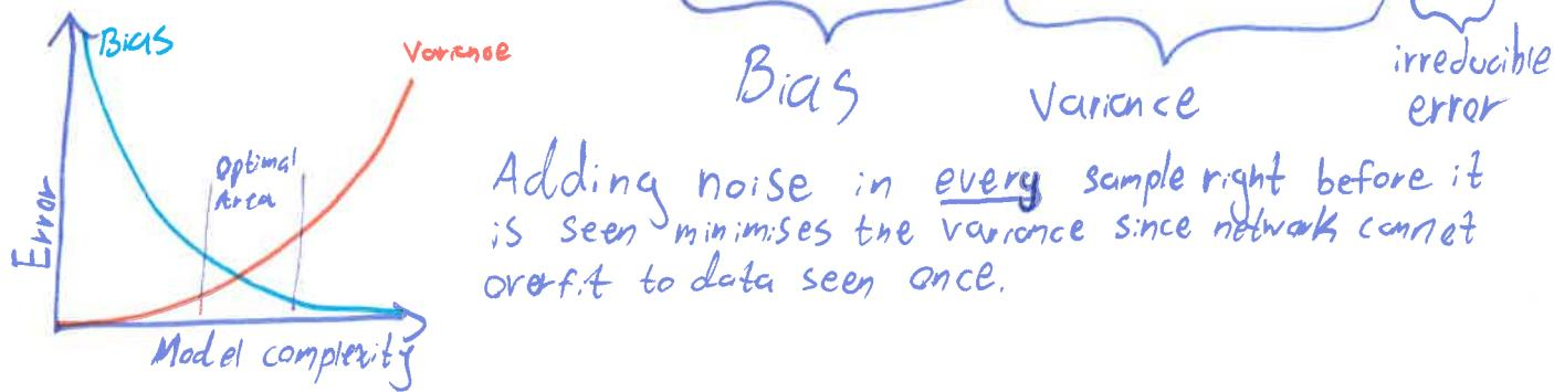
Adding noise in every sample right before it is seen minimises the variance since network cannot overfit to data seen once.
