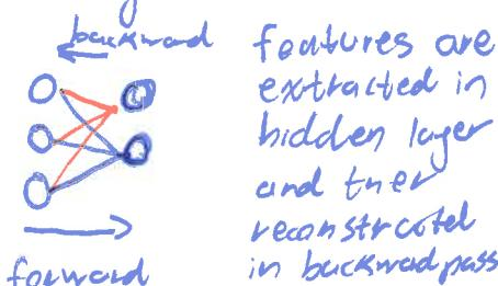
Features are extracted in hidden layer and then reconstructed in backward pass
